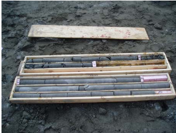
Photo 9- Coring of Jet-Grouted columns
